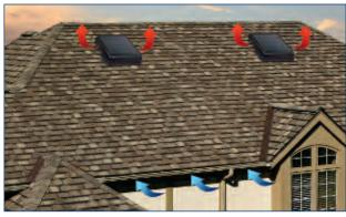
Hot, stale attic air is removed through the High-Power Solar Roof Vents. Fresh air is drawn into your attic through your soffit (or other) intake yents
