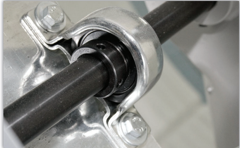
Rubber mounted shaft bearings
